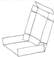
Figure 4 -Folding and glueing seat cushion and base
